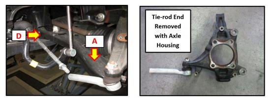
**IMPORTANT NOTE: ALWAYS** use new wheel bearing mounting flange bolts, strut self-locking nuts, axle nuts, and tie rod end nuts during assembly. Be sure to torque these items to the correct specification.
