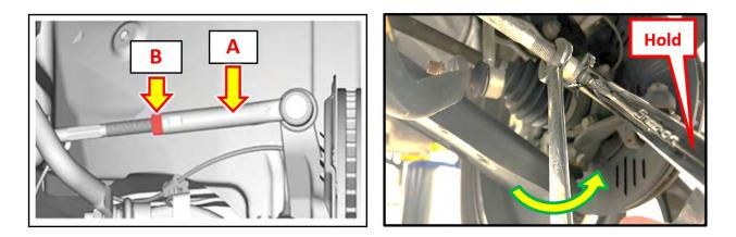
**STEP 3:** While holding the steering gear box boot (**C**) and **CAREFULLY** preventing it from turning, loosen the tie rod (**D**) with a 14mm wrench. Take note of the number of rotations during removal and apply the rotation number to the new part installation. This will help save time during the alignment. Use **CAUTION** when performing this STEP to ensure the steering gear box boot does not twist/and or rotate.
