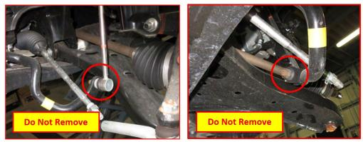
**Tip 2:** Even with usage of a recommended ball joint separator tool (shown below), there can be difficulty separating the tie rod end from the axle housing. This is caused by possible deformation of housing/tie rod from exceeded torque limits during installation. **ALWAYS** use eye protection when attempting to apply this method. If there is difficulty found when removing/separating the tie rod end with the axle housing, follow the procedures outlined on the next page.
