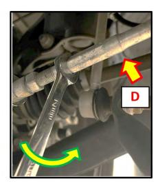
Once the tie rod end is removed from the tie rod, proceed to further removing the axle carrier.
