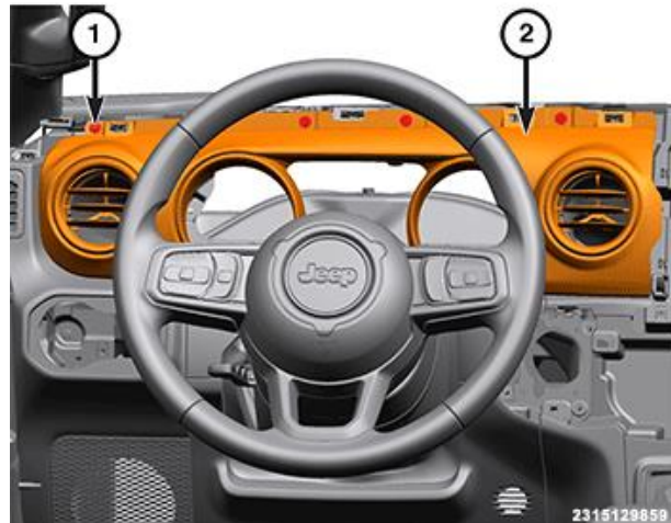
Figure 7 – IPC Bezel Screws
