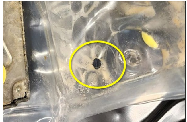
Cover pinched, resulting in puncture.
