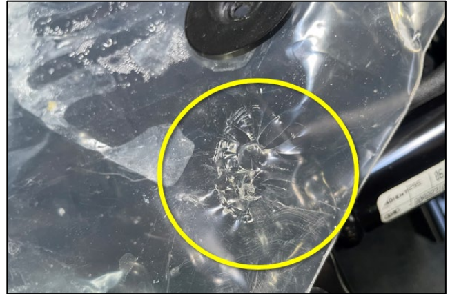
Cover pinched, resulting in puncture.
