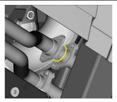
6. Install the 2 new seals (WHT004894) and the 4 new screws (N10558102) by following the removal procedure in reverse order.
