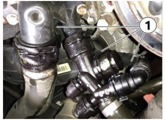
• NOTE: The new coolant line PN 11 14 7 827 410 is routed in a different location than the original line (1)
