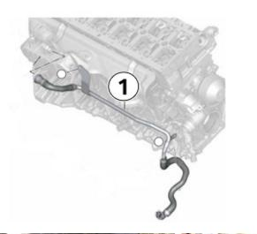
• Replace the coolant pipe from the Auxiliary EGR cooler to the coolant pump distribution block (1)
