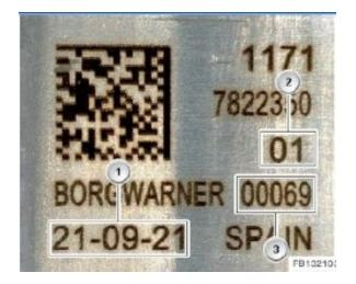
**Hint:** Record or take a photo of the following numbers on the new EGR cooler before installation (1, 2 and 3). These numbers will be required later to register the new cooler in ISTA.
