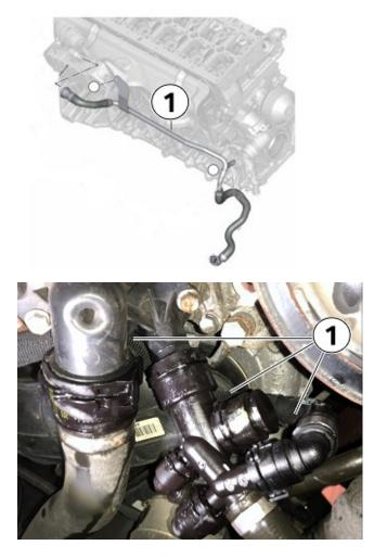
• Replace the coolant pipe from the Auxiliary EGR cooler to the coolant pump distribution block (1)
