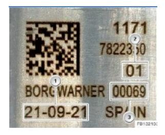
**Hint:** Record or take a photo of the following numbers on the new EGR cooler before installation (1, 2 and 3). These numbers will be required later to register the new cooler in ISTA.
