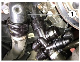
NOTE: The new coolant line PN 11 14 7 827 410 is routed in a different location than the original line (1)
