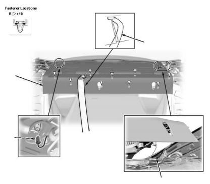
9. Cut the seat belt webbing of the center seat belt to destroy the bad seat belt.
