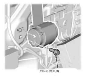
13. Install the new rear center seat belt assembly and torque the bolt to 39 N.m (29 lb-ft).
