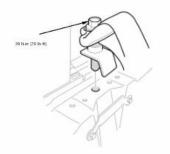
12. Remove the rear center seat belt assembly.
