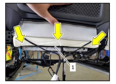
• Ensure seat foam <arrows> is fully engaged over the rear of the seat pan <1>.
