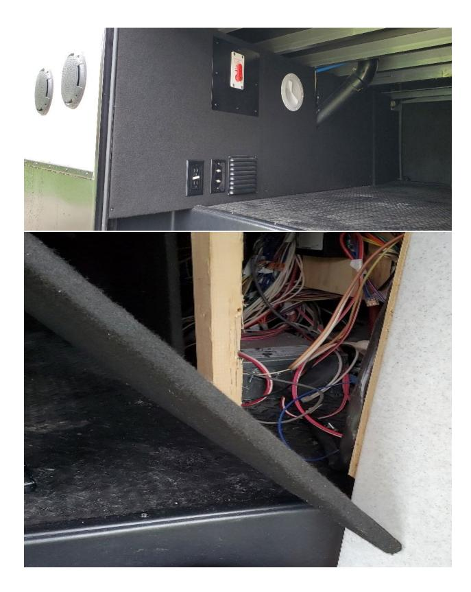
3. Once access has been gained to transfer switch, remove cover using a 1/4" socket to loosen set screw
