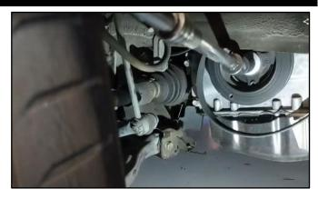
5. Show the engine being cranked and torque specification exceeding 94 lb.ft. torque.
