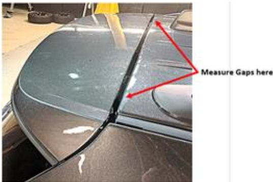
Figure 3 – Gap from Spoiler to Roof
