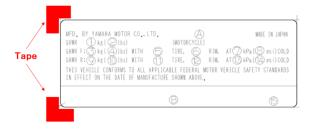
7. Gently peel the Vehicle Certification Label from the frame. Use a heat gun to ease the removal process. Once the incorrect label has been removed, <u>please destroy it before throwing it away</u>. Clean any remaining adhesive with soap and water or a detergent-based cleaner. Wipe the area using a dry rag.
