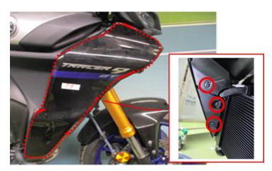
4. Remove the right side cover by pulling the three projections from the grommets.
