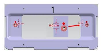
4. Using a 5mm drill bit, drill 2 new holes exactly 8mm directly above the metal bushings as shown to the left.
