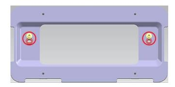
2. Inspect the 2 mounting screws of the rear license plate bracket as shown to the left.
