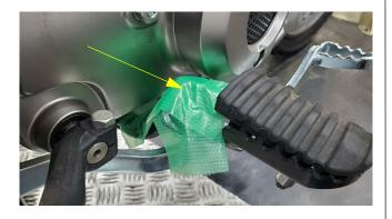
Remove the four flange bolts [1] from the step bar [3].
