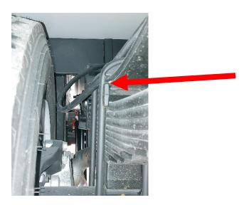
2. Attempt to pull excess slack of hose to rear of motorhome as shown in below photos, eliminating slack and potential for sagging. If excess hose is present, securement will be required. Use additional p-clamps to secure any excess that may be present.
