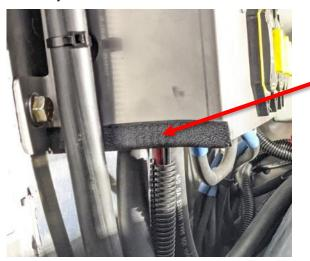
Install trim lock to the bottom left corner of the CB assembly
