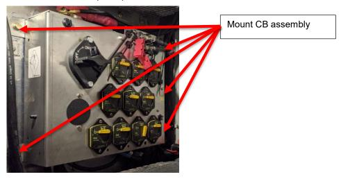
36. Using tie cable with mount, MCI P/N: 19-11-3472, and tyraps to secure the battery ground to the left side of the CB assembly.
