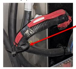
Remove BT-P162 tyraps on battery cables.
