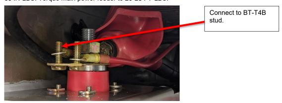
40. Connect the fuse block C ring terminal (Wire ID 0047) to the 24V SW stud (BT-T4C) on the circuit breaker busbar, MCI P/N: 7L-8-5055, using lock washer, MCI P/N:19-2-37, and nut, MCI P/N: 19-3-32. Torque stud to 65 IN-LBS. Spray 3 studs with anti-corrosive spray, MCI P/N: 23-02-0119.
