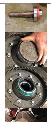
11) Carefully remount the hub-rotor onto the spindle by hand.
