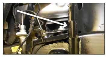
14. Install the new upper control arm to the vehicle using the **new provided 14mm bolts, washers, and nuts and using the provided thread locker.** Run the bolt with a washer from the inside out of the strut bucket outwards. Apply thread locker and fasten with a washer and nut on the outer bushing washer surface. Do this for the front and rear control arm mounts. Snug up hardware.
