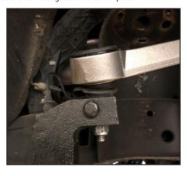
22. Reattach the tie rod to the knuckle. Torque the tie rod end nut to 44 ft-lbs.
