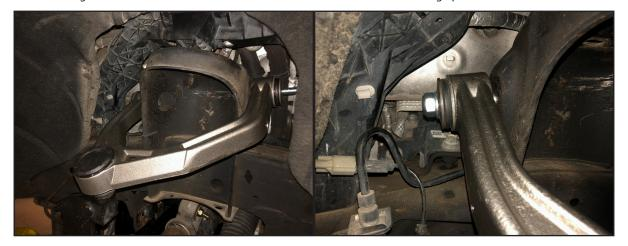
15. Attach the ball joint on the new upper control arm to the knuckle. Snug up ball joint using the OE nylock nut, **but do not torque down**. The upper ball joint will be removed from the knuckle later so that the strut can be installed.
