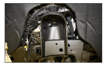
13. The new replacement control arm assemblies have a larger profile than the OEM assemblies. They are also designed with a wider range of available travel. Due to these unique differences, the tab on the side of the strut bucket must be removed to avoid interfering with the proper function of the new control arm assembly. Cut the tab from the side of the strut bucket as shown below.
