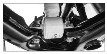
10. Remove the three nuts attaching the strut to the frame. Remove the strut from the vehicle. DO NOT remove the center strut rod nut.
