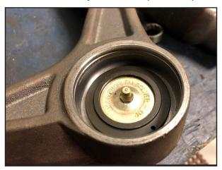
3. Lightly grease the O-ring and reinstall the ball joint cap by pressing firmly on the cap to seat it into the upper control arm.
