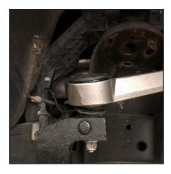
16. Important: Set the ride height from the fender lip to the center of the hub at 28". Using a torque wrench on the inside of the strut bucket and a wrench on the outside bushing to prevent the nut / bushing from moving, tighten the control arm hardware to 148 ft-lbs. This will ensure the rubber bushings are tightened to the right position and not put preload in the rubber bushings. DO NOT spin the "bushing side" hardware when tightening, only tighten from the inside "frame side".
