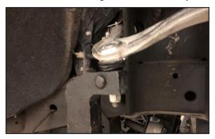
9. Remove the two lower strut bar pin bolts. Lower the control arm with the jack so there is enough room to remove the OE strut assembly with the strut spacer still attached.
