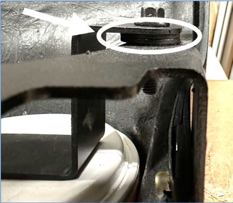
Figure 16: Two washers per screw
