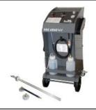
Brake Filling and Bleeding Equipment -VAS6860-(or equivalent)
