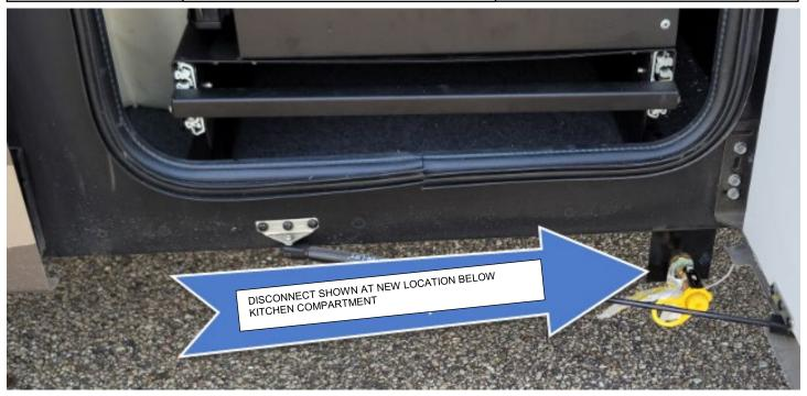
NEW DISCONNECT LOCATION SHOWN ABOVE AT FRONT SIDE RIGHT BELOW COMPARTMENT. USE NEW QUICK DISCONNECT HOSE THAT WAS PROVIDED WITH PARTS KIT TO CONNECT TO RANGE.
