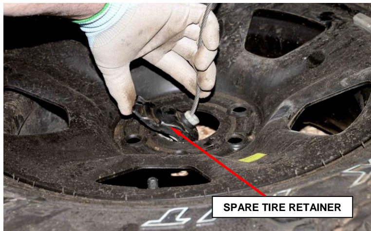
Figure 7 – Spare Tire Winch Release
