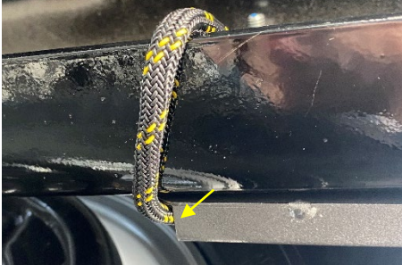
Bottom view of the wires around the frame and into the fender guide.
