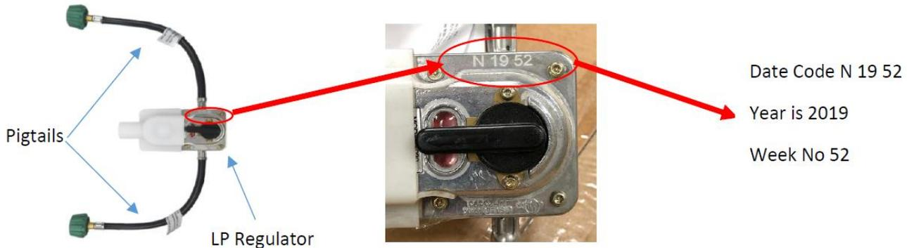
2. File a claim for inspection only if the unit does not have a Winntec model #6020 LP regulator or if the date code stamped into the regulator is not 18 XX, 19 XX or 20 XX. Only replace regulators with date codes 18 XX, 19 XX and 20 XX.
