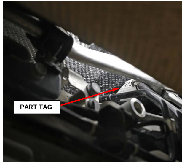
Figure 2 – Part Tag on Fuel Line
