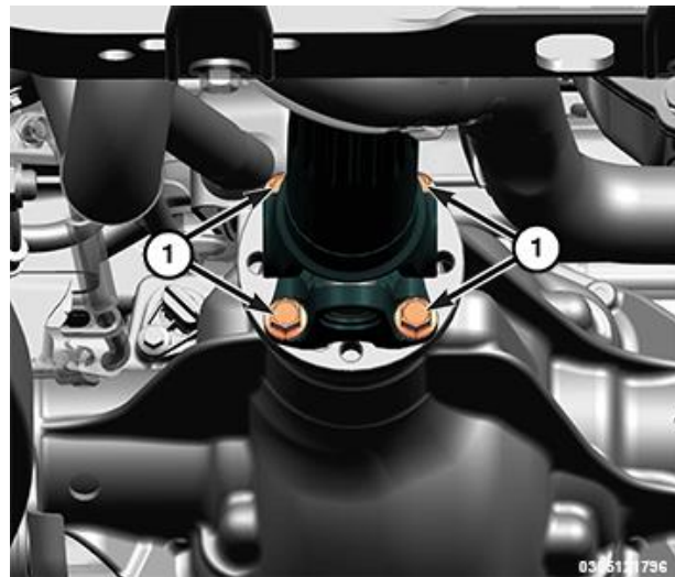
Figure 15 – Front Driveshaft Bolts
