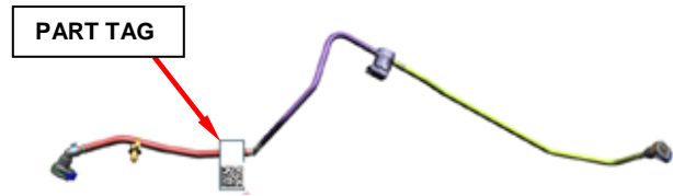
Figure 1 – Part Tag on Fuel Line
