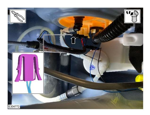
3. The 2 fuel filter ground wires must then be spliced into the fuel pump driver module wiring harness. If required, (see TOPIx Workshop Manual section 418-02: Wiring Harnesses - Description and Operation - Wiring Harness).
