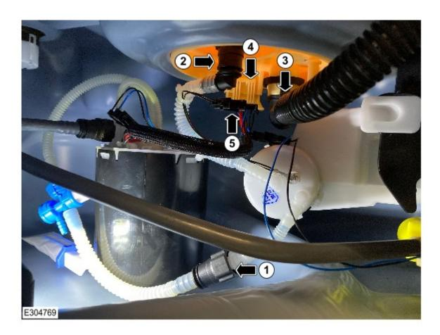
Make sure the fuel hose is positioned as shown, facing away from the fuel tank flange electrical connector.
