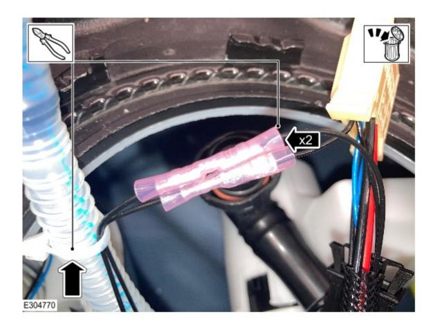
2. To install the new fuel tank flange assembly, remove and discard the male electrical connector from the new fuel filter.
