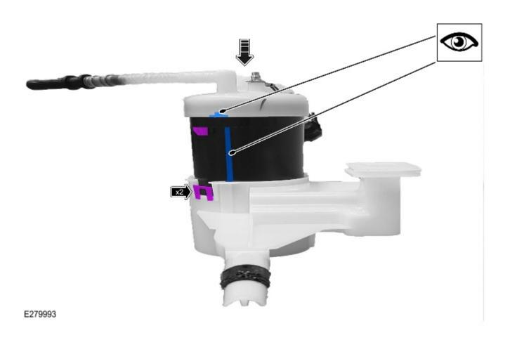
3. Install the bracket and fuel filter assembly into the fuel tank, an audible click will be heard when the bracket and fuel filter assembly is correctly installed. Each illustration shows the installation from different angles.
