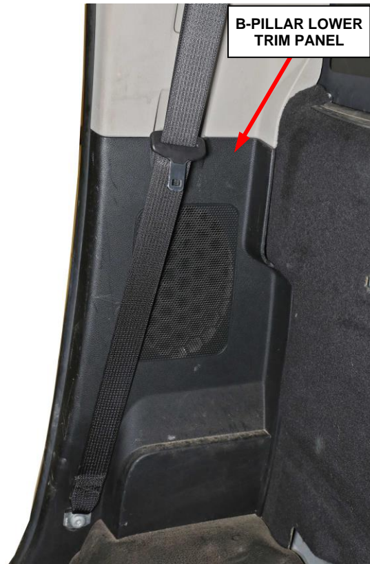
Figure 3 – B-Pillar Lower Trim Panel
