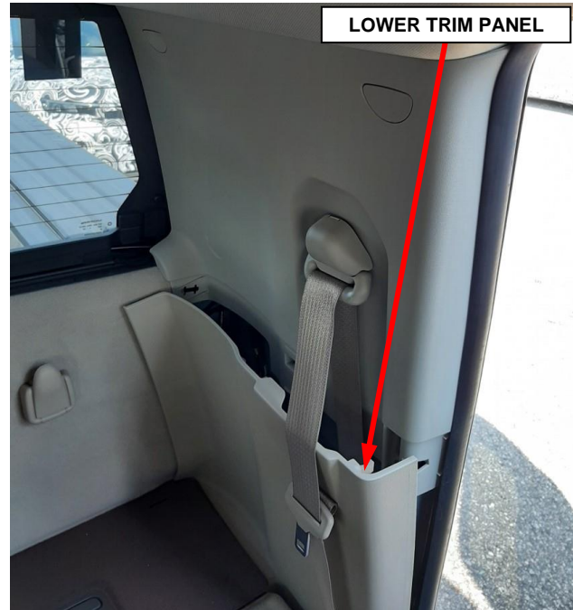
Figure 61 – C-Pillar Lower Trim Panel
