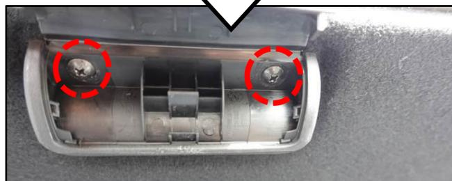
2. Remove the trunk lid trim by referring to the "Body (Interior and Exterior) → Trunk Lid → Trunk Lid Trim → Repair procedures" in the applicable Shop Manual on KGIS.
