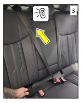
**Step 3)** Slowly retract the webbing all the way back into the seat belt retractor while the seat belt remains buckled. You will hear a ratcheting sound.
