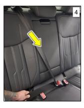
**Step 4)** Pull on the seat belt and verify it is locked and cannot be pulled out of the seat belt retractor.
