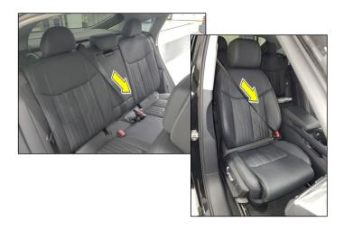
Check the Automatic Locking Retractor (ALR) function on the seat belts according to specified criteria, and replace if necessary.
