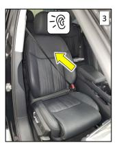
**Step 3)** Slowly retract the webbing all the way back into the seat belt retractor while the seat belt remains buckled. You will hear a ratcheting sound.
