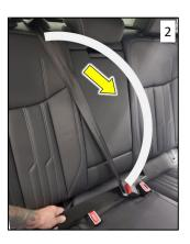
**Step 2)** Pull webbing all the way out of seat belt retractor to activate ALR.
