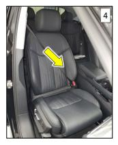
**Step 4)** Pull on the seat belt and verify it is locked and cannot be pulled out of the seat belt retractor.
