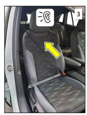
**Step 3)** Slowly retract the webbing all the way back into the seat belt retractor while the seat belt remains buckled. You will hear a ratcheting sound.
