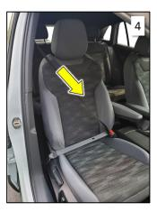
**Step 4)** Pull on the seat belt and verify it is locked and cannot be pulled out of the seat belt retractor.
