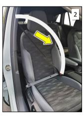
**Step 2)** Pull webbing all the way out of seat belt retractor to activate ALR.
