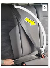
**Step 2)** Pull webbing all the way out of seat belt retractor to activate ALR.
