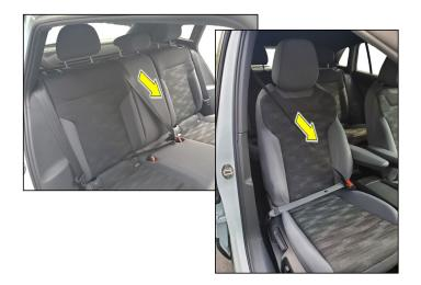
Check the Automatic Locking Retractor (ALR) function on the front passenger and rear center seat belts, and replace if necessary.
