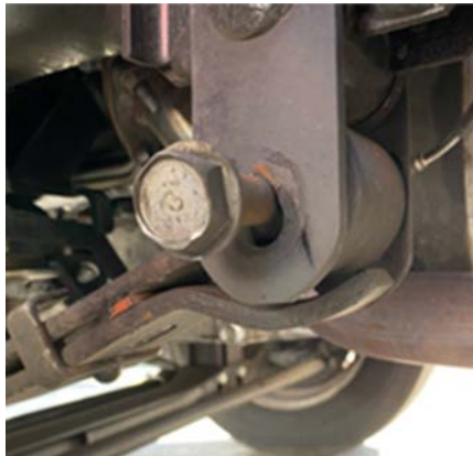
Example of damage on shackle
