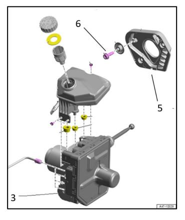
Install the new brake pressure unit in the reverse order of removal:
