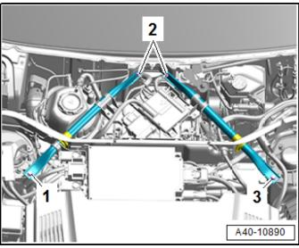
Remove the bolt <3> and nut <2> (left side) and remove the left (driver side) tower brace.
