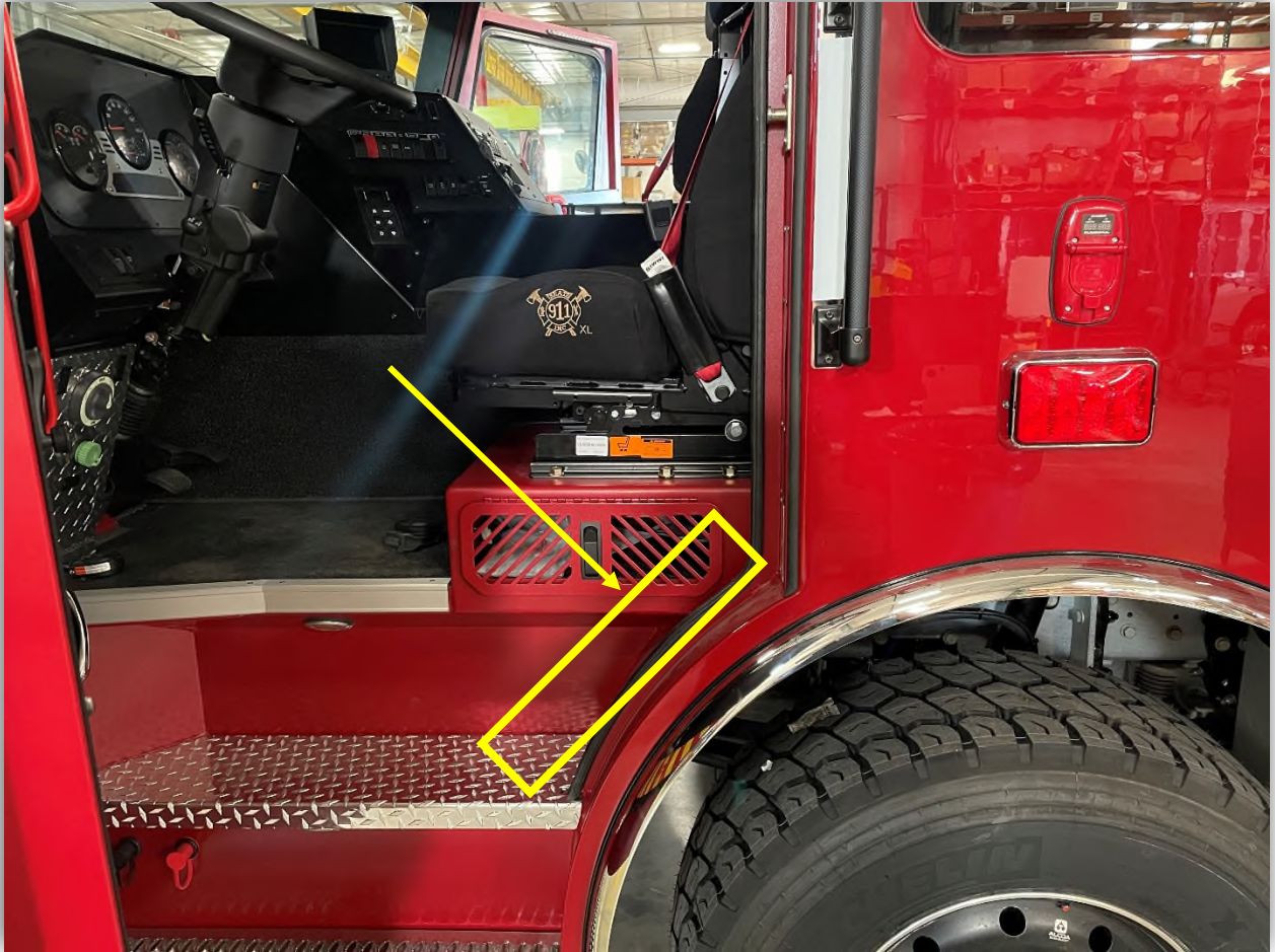
Image 5: Wheel Well VIN Plate Installation Location.
