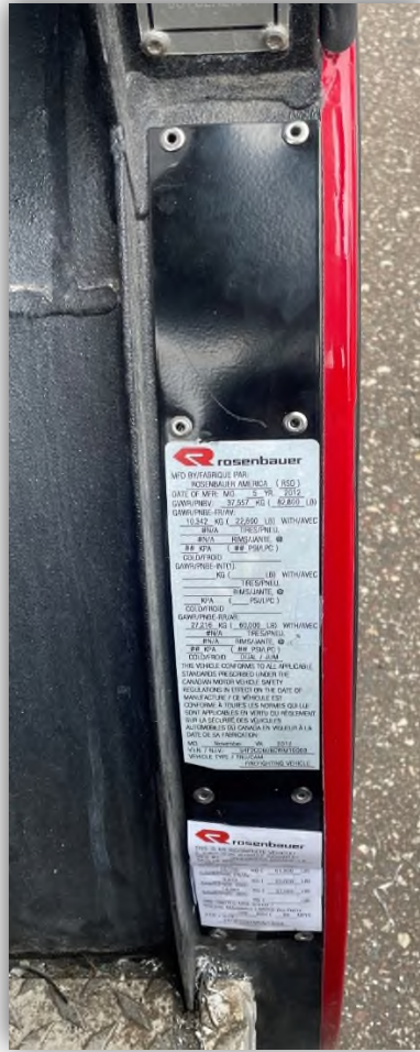
Image 9: Completed VIN Plate installation
