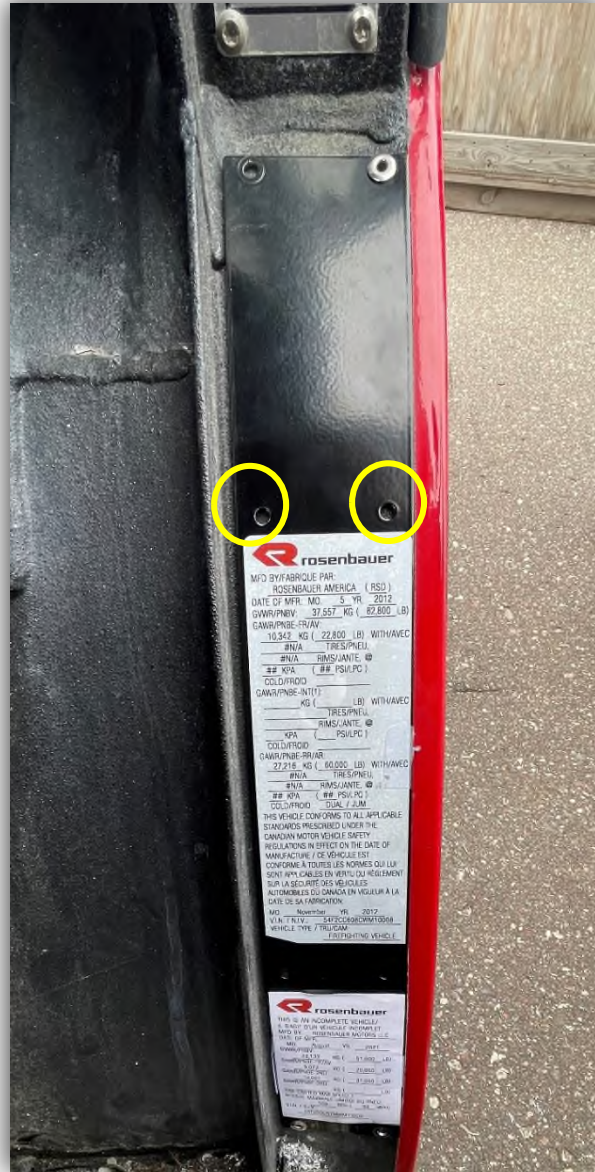
Image 8: Second set of holes and rivets to be installed.
