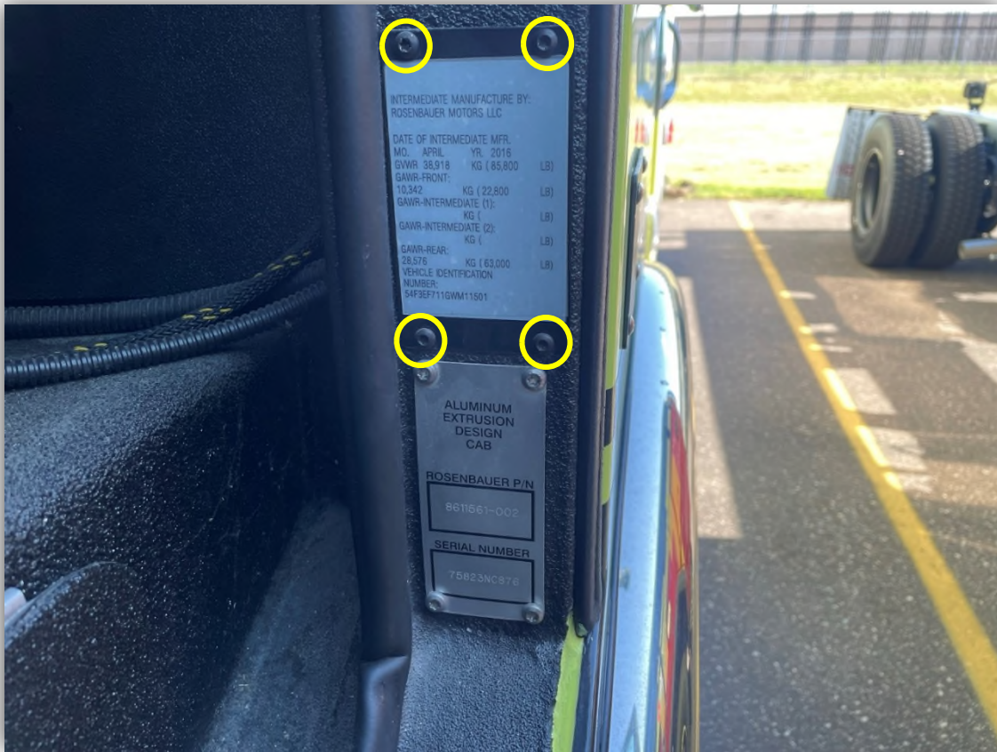
Image 4: Incomplete Vehicle Tag Removal from B-Pillar location.
