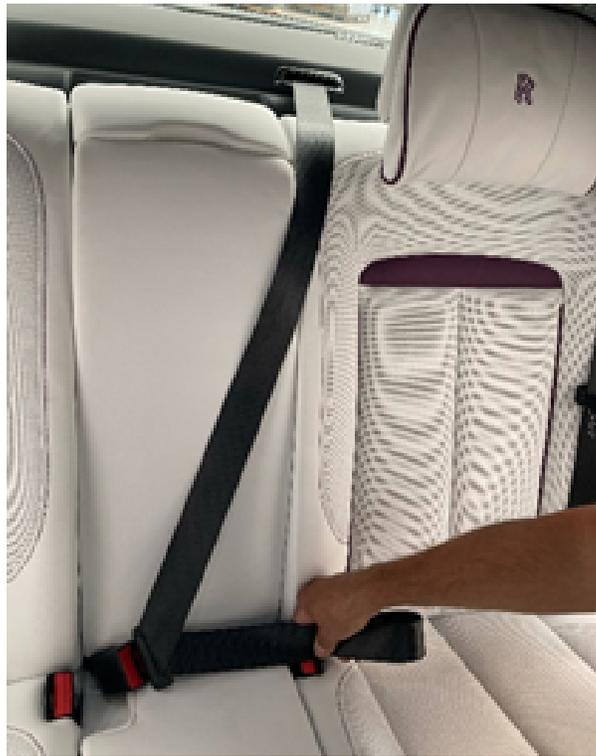
Step 2 Pull the seat belt/webbing all the way out of the retractor to activate the ALR.
