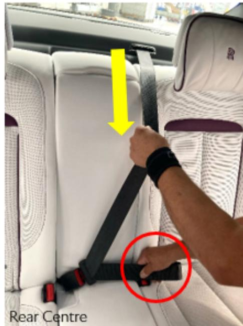
Is the seatbelt locked so the webbing cannot be pulled out of retractor in Step 4?
