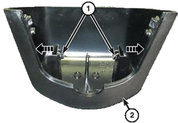
Figure 3 – Lower Mirror Trim Tabs
