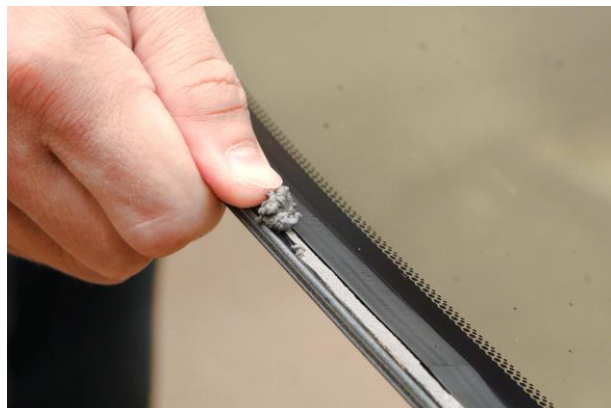
Figure 20 – Remove Lace Molding Adhesive
