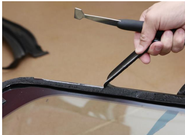
Figure 19 – Remove Old Lace Molding
