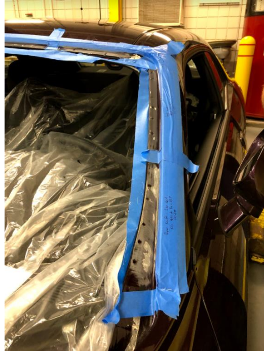
Figure 25 – Protect Adjacent Surfaces
