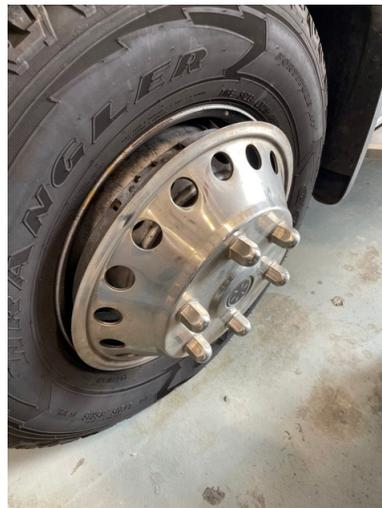
2. Inspect the valve stems for any signs of damage or wear due to contact with the wheel liner. If damage is found, please contact Wayfarer warranty department at 205-487-4710.
