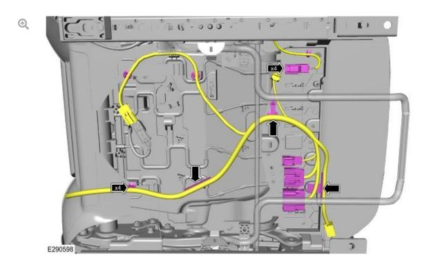
Release and move aside the wiring harness.
