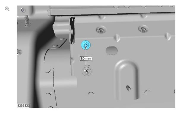
Install a new body ground stud (LR149837) 50 mm above the existing ground stud (G4D178) (see TOPIx Workshop Manual section 501-25A: Body Repairs General Information - General Procedures - Body Earth Stud Repair).
