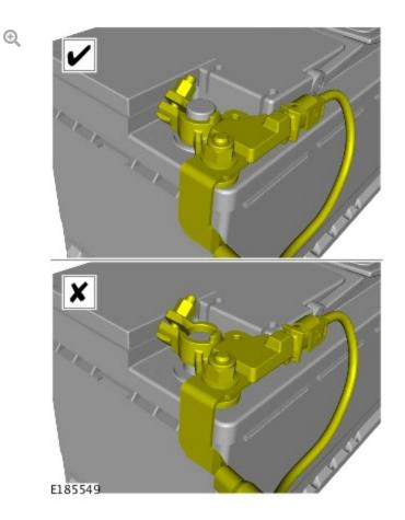
Connect the startup battery ground cable (see TOPIx Workshop Manual section 414-00: Battery and Charging System - General Information - Specifications).
