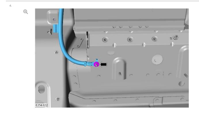
Remove the startup battery ground cable from the body ground stud (G4D178).
