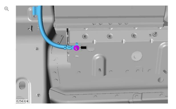
Install the startup battery ground cable to the new body ground stud.
