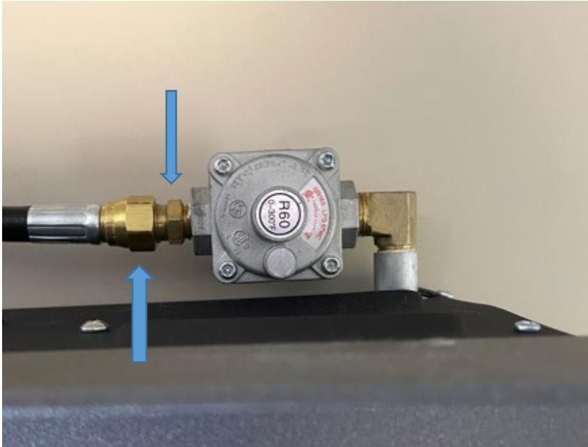
Use a 3/4" and 5/8" wrench to tighten the LP connection.
