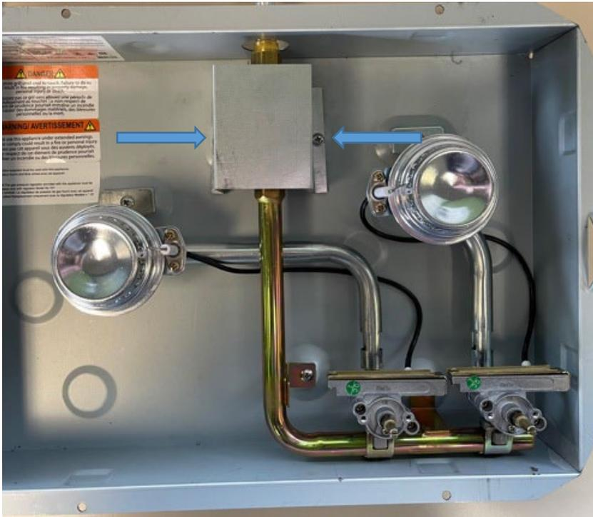
Remove the screws from the shield using a screw driver.
