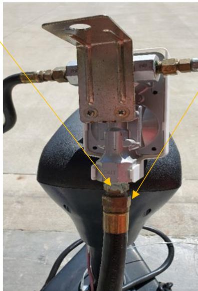
6. Once regulator is removed, using a 3/4" wrench remove the brass fitting at the bottom of the old regulator that the LP line connects to and install on the new regulator with new pipe compound or thread tape. DO NOT USE PIPE COMPOUND OR THREAD TAPE ON FLARED FITTINGS
