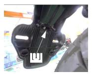
2. Remove the defective Reflector and install the new Reflector [2] by aligning the Reflector pin to the fixing hole. Tighten the new U-nut to 13 in-lbs (1.5 N.m).
