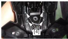
6. Remove the License Light Bracket from the Rear Fender A.
