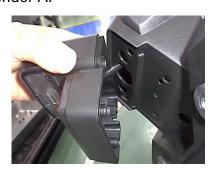
7. Remove the U-nut [6] from the License Light Bracket and remove the defective Reflector.
