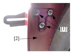
2. Remove the License Plate Bracket [1]from the Rear Fender Comp [2].
