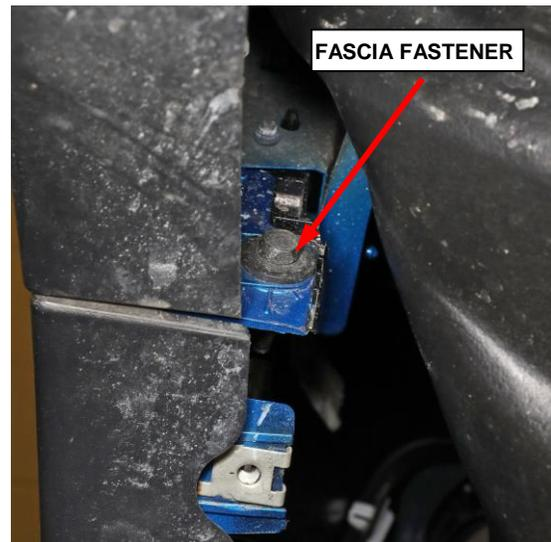
**Figure 9 – Fascia to Fender Fasteners**
