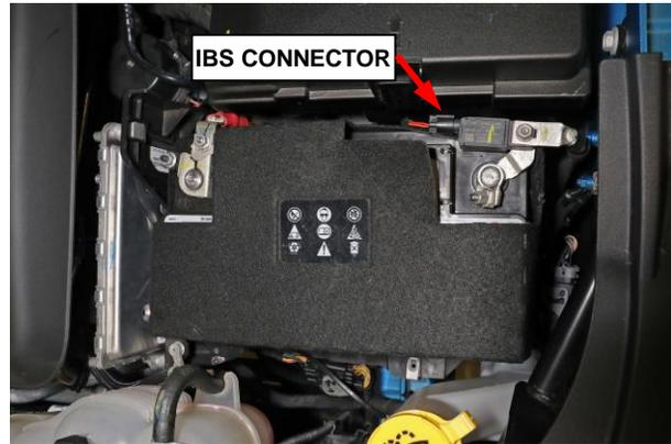
**Figure 4 – Battery IBS Connector**
