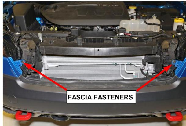
**Figure 6 – Fascia Fasteners**
