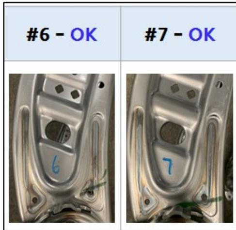
5. If a front seat back does not meet the inspection criteria, replace the front seat back frame assembly.
