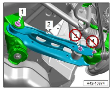
The nuts at connection <1> of <u>both</u> rear lower control arms <2> will be replaced.
