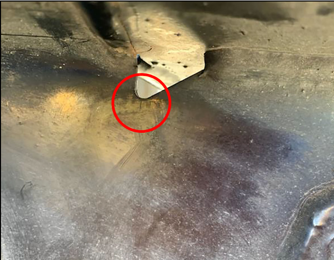
Example: Vertical surface crack – not contained within template (refer to template on next page)
