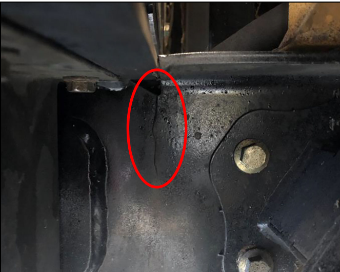
Example: Vertical surface crack – not contained within template (refer to template on next page)
