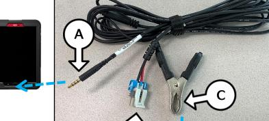
2b. Connect the knocking sensing connector (B) of engine vibration inspection harness to the knock sensor connector on the vehicle.
